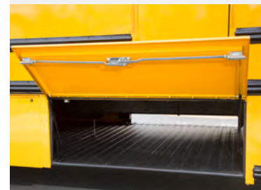
Optional underbody pass-through storage adds capacity of up to 129 cubic feet.
