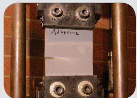
D ADHESIVE AFTER: Adhesive after pull test. Adhesive at 2" overlap, metal tears at an average of 14,475 lbs. (joint did not break).
