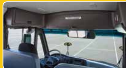
The cockpit features increased overhead storage space and improved interior rearview mirror placement.
